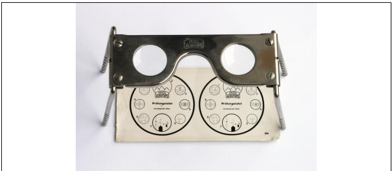
Figura 4. Stereograf militar portabil ( http://en.wikipedia.org/wiki/File:Pocket_stereoscope.jpg )
